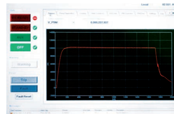
TINE based control system displaying a pulse.
