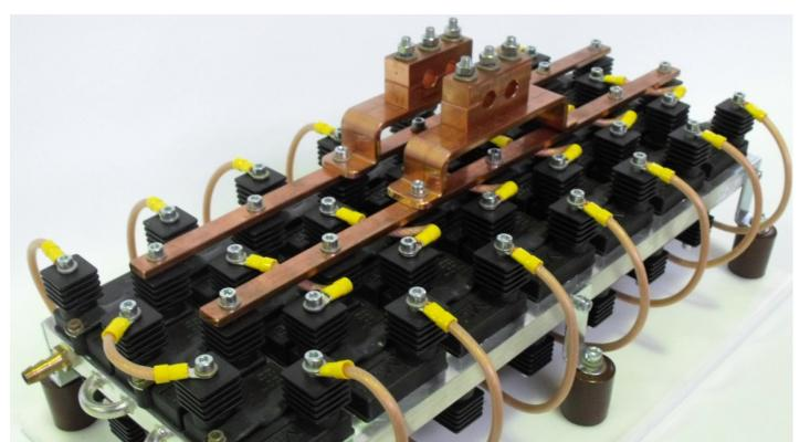
Klystron Replacement Dummy at Modulator Commissioning Site
