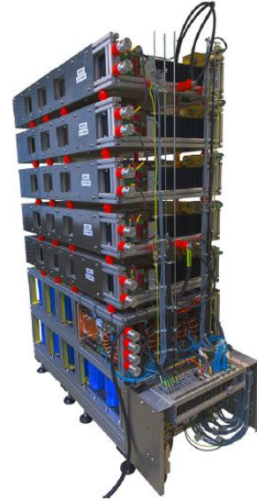
Fig. 3. Prototype of a unipolar current source with a maximum output current of 1.4 kA and voltage of 5.5 kV.
